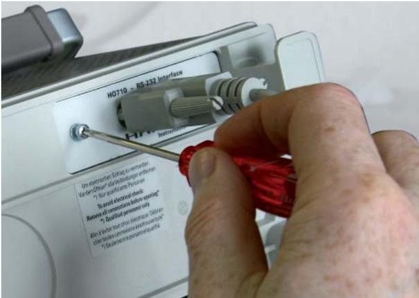
5.1.1 Remove both fastening screws.
