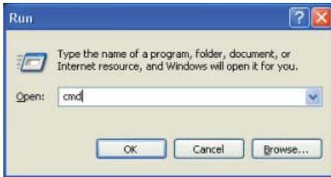
It opens an input window. After the input character you give to confirm the instruction "ping 192.168.10.10" (in the represented example the Ethernet interface of the oscilloscope has the IP address 192.168.10.10) and confirm the input with Enter.
