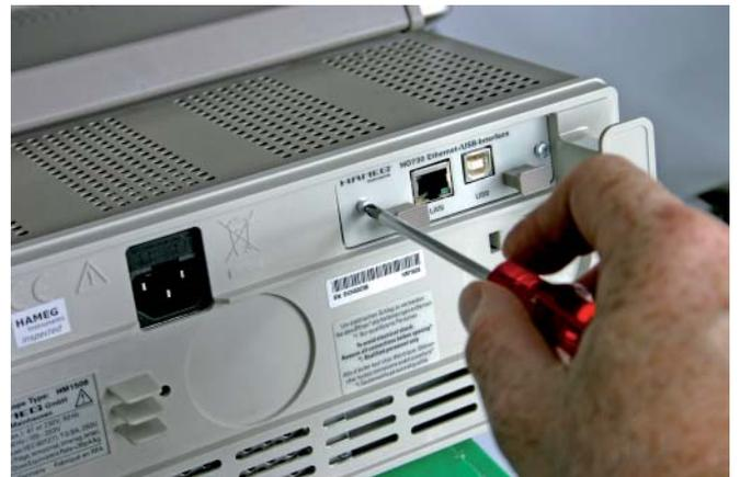
5.2.2 Fit the interface with the fastening screws previously (item 4.1.1) removed.
