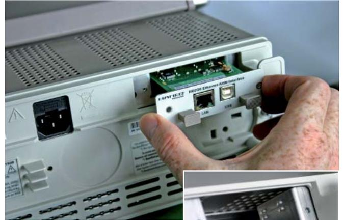
5.2.1 Insert the interface H0730 in the opening in such a way, that the PCB will be inserted in the guides - visible on both sides - and push it in completely.
