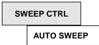
Define whether a sweep is to be carried out, whether the sweep is specified by parameters or a list and whether the sweep is to be continued automatically or manually via rotary knob. Switch to AUTO SWEEP. The panel shows some additional lines in which the sweep parameters are to be specified:
